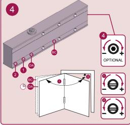
DABC VALVES NOT STANDARD, THESE ARE OPTIONAL FOR UNINSULATED STEEL DOORS IP.95M MUST BE USED. THE PINION BOLT MUST BE TIGHTENED TO 12NM.
