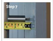
Using a tape measure check the amount which will need to be removed from the bolt.
