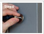
Insert the bolt into the grommet and screw in until it no longer moves.
